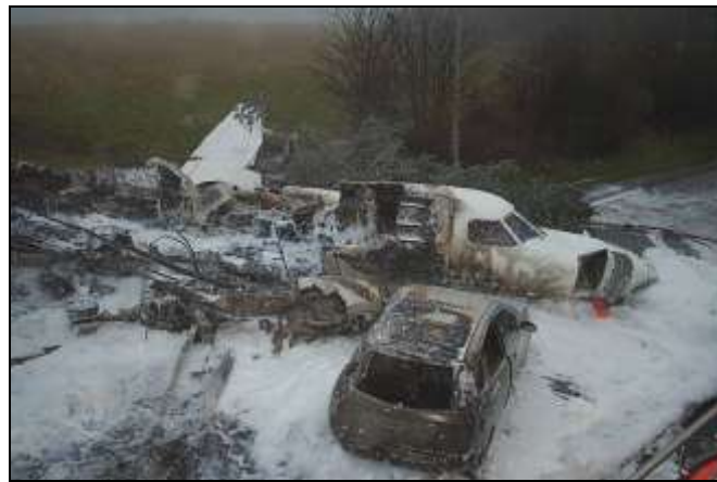
The foam covered wreckage of the Metro on the road
